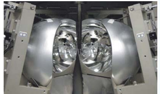
傾斜鏡型赤外線集中加熱炉 Tilting Mirror Type Infrared Convergent Image Furnace
